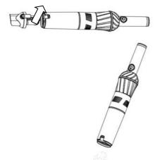
2, Rotate the dust cup to the left and remove the dust cup.
